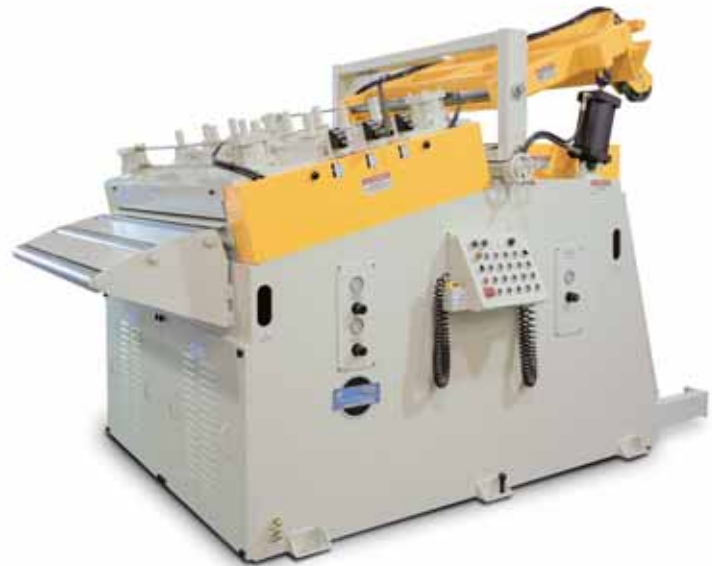
■ 305 Series straightener shown with optional peeler/threader/hold down station, single row of back-up rollers and digital upper roll height indicators.
